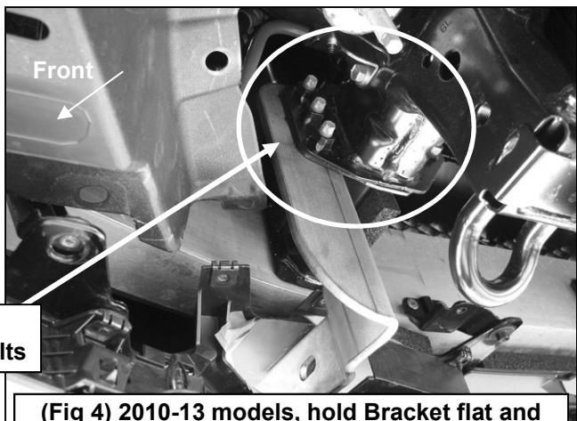
(Fig 4) 2010-13 models, hold Bracket flat and
