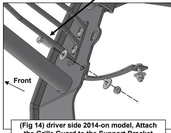
(Fig 14) driver side 2014-on model, Attach the Grille Guard to the Support Bracket
