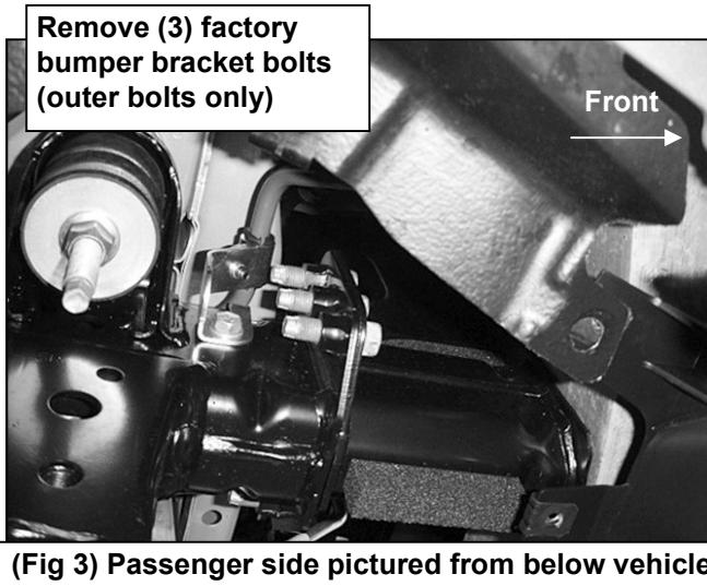
(Fig 3) Passenger side pictured from below vehicle
